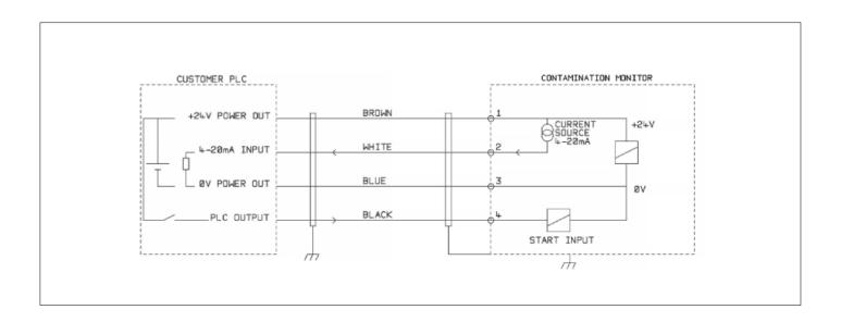
The cable + connector needs to be a shielded 4way, A-coded, female pin type. An example could be TE 2273099-1. Alternatively a rewireable type can be used.
