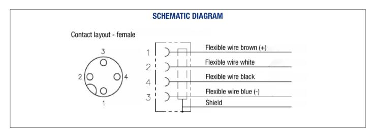
The OV is connected internally to the case as well as the shield.
