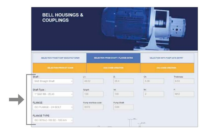
Then, Shaft / flange technical drawing will appear, with data taken from the database.
