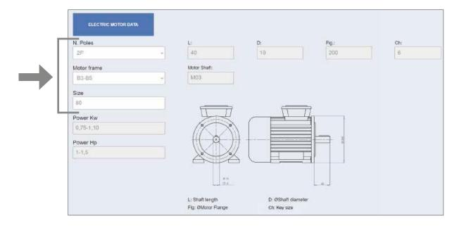
Once above data are input, fields related to motor sizes and technical drawing will appear, with data taken from the database.
