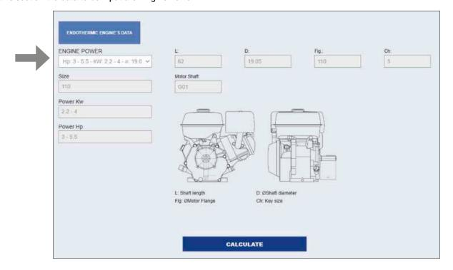
Once above data are input, fields related to motor sizes and technical drawing will appear, with data taken from the database, created from motor manufacturer official data.
