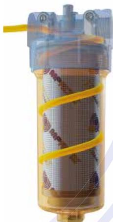
High flow rate thanks to the head geometry: the oil enters in the filter element in a spiral flow and spreads more effectively inside the filter element for greater longevity.
